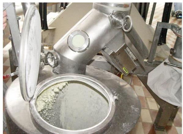
*Figure 3: NIR-Online sensor installed at the bottom of a spray dryer. Monitored parameters include moisture and fat.*
